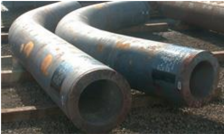
Induction bends on thick-walled pipes
